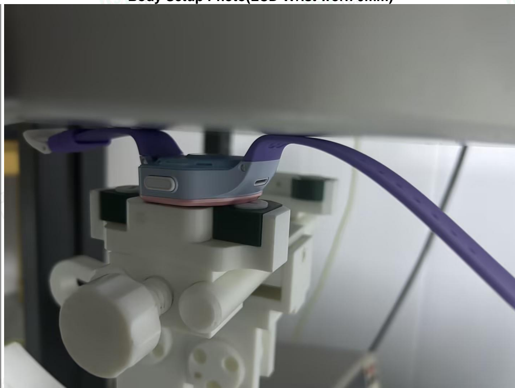
Body Setup Photo(LCD Wrist worn 0mm)
